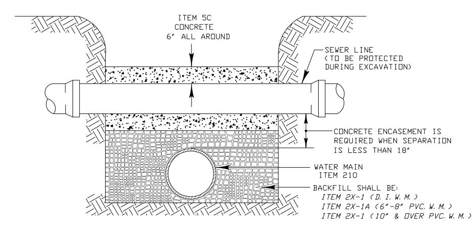
NOTE: CROSSING IS TYPICAL. OTHER TYPES OF WATER/SANITARY SEWER MAIN CROSSINGS SHALL BE TREATED IN A SIMILAR MANNER, A. O. B. E.
