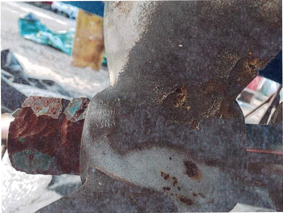
Example of galvanic corrosion on a Boat Propeller and Nut.
