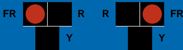
5. Alternating Flashing Red During Pedestrian Clearance Interval
